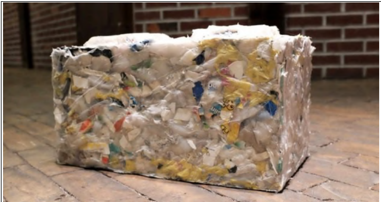
Figure 11: Picture of a construction brick made of plastic waste
